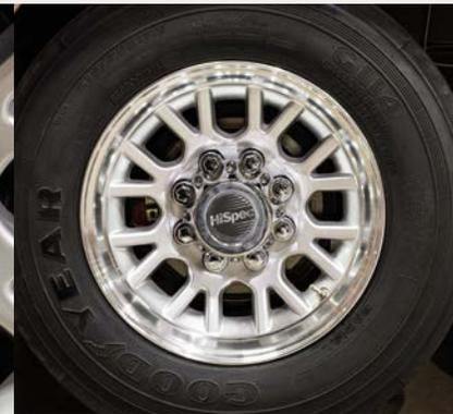
Heavy-duty 17.5" Goodyear® tires provide increased load capacity while staying cool on long hauls. We use truck tires, not RV tires, to ensure better performance and peace of mind.
